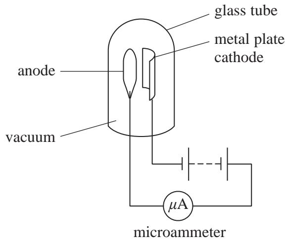
When light is incident on the cathode, the microammeter shows a current.
