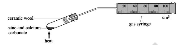
A mixture containing 0.27 g of powdered zinc and 0.38 g of powdered  $CaCO_3$  was heated strongly for two minutes. The volume of gas collected in the 100 cm<sup>3</sup> syringe was then measured. The experiment was then repeated.
